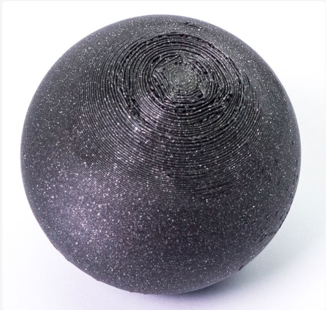
Printing a sphere cut into two hemispheres, which are then glued together.
