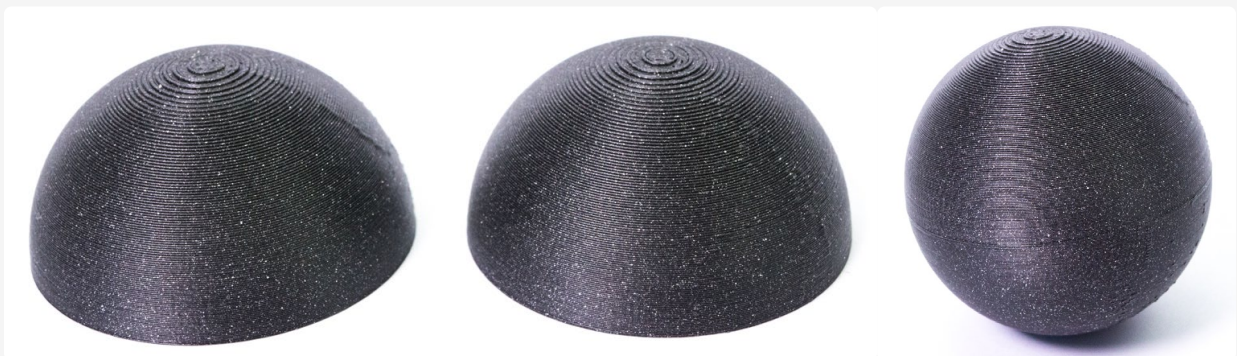
Printing a sphere cut into two hemispheres, which are then glued together.
