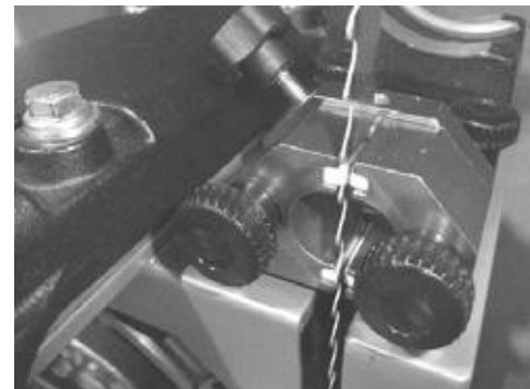
Side guides adjusted with ceramic just behind the gullet
