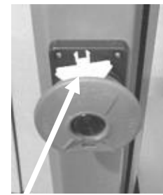
Start/stop with safety removed
