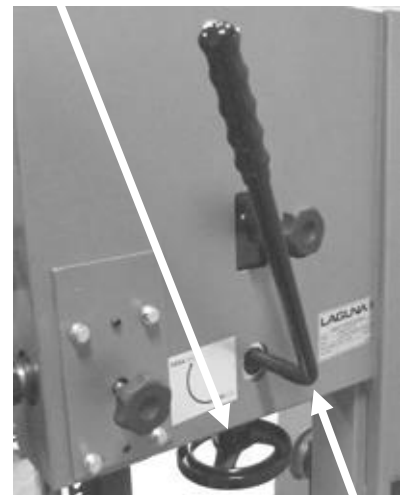
Quick action blade tension lever (activated)
