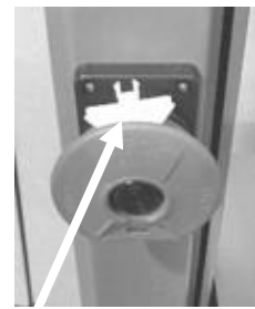
Start/stop with safety removed
